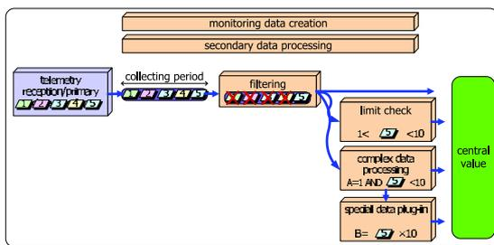
Figure 6: Secondary data processing (filtering)
